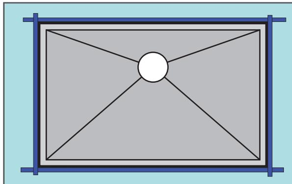
3. Remove the sink from the counter top leaving the blue tape guide for installation.
